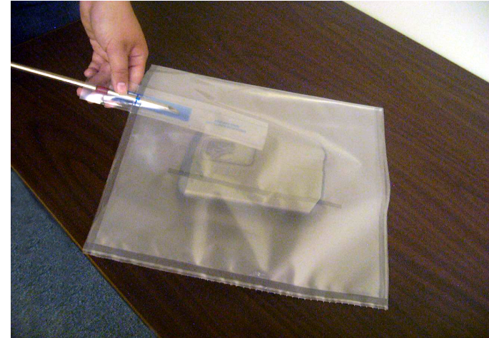
2. Insert inflator into the blue valve.
