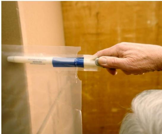
**2. Insert inflator into blue valve. Place finger on valve to hold in place.**
