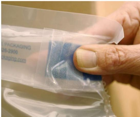
**5. Fold over valve while firmly pressing down.**
