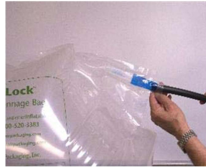
Step 2. Insert deflator tube into blue valve.
