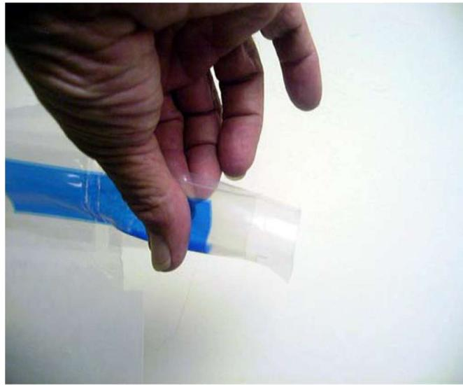
Step 1. Open valve with blue side facing you, by rolling between thumb and index finger.
