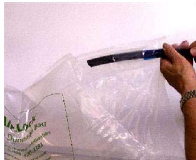
Step 3. While holding valve in left hand, push deflator completely into valve.
