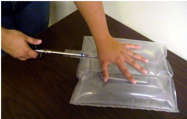
3. Press trigger, allowing air to flow into the sleeve.
