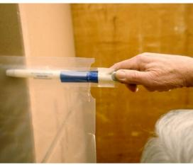
2. Insert inflator into blue valve. Place finger on valve to hold in place.
